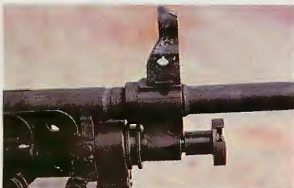
ABOVE: SAW front sight and gas regulator. BELOW: Textured, curved butt pad.
